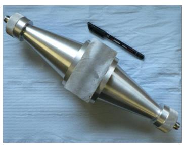
Figure 5.23 Biconical transmission line arrangement
