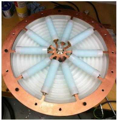
Figure 4.9 130  $\Omega$  resistor, made from ten identical aqueous 1.3 k $\Omega$  resistors radially mounted in parallel. When connected to the output of the Blumlein PFL generator, the empty space is filled with transformer oil.
