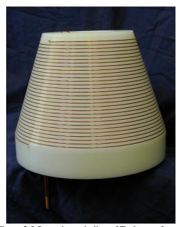
Figure 2.5 Secondary winding of Tesla transformer
