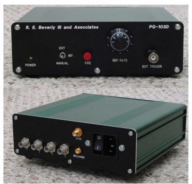
Figure 6.5 PG-103D front panel and rear panel showing four channel unit [6.6]
