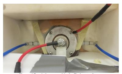
Figure 6.7 switch mounted in the Tesla transformer
