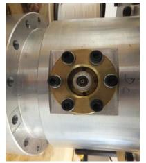
Figure 5.4 Voltage sensor mounted on coaxial load
