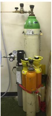
Figure 6.13 Sulphur Hexafluoride arrangement
