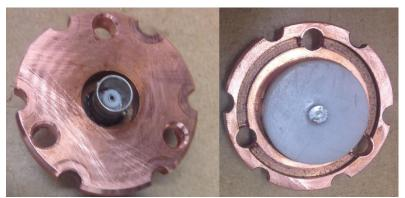
Figure 5.3 Voltage sensor for oil-filled Blumlein PFL
