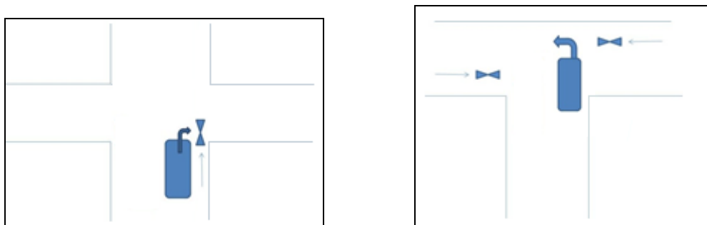
Figure 3 Critical PTW scenarios (a): PTW being hit by a vehicle heading in the same direction and then turning across the path of the PTW; (b) vehicles pulling out from intersections into the path of the PTW
