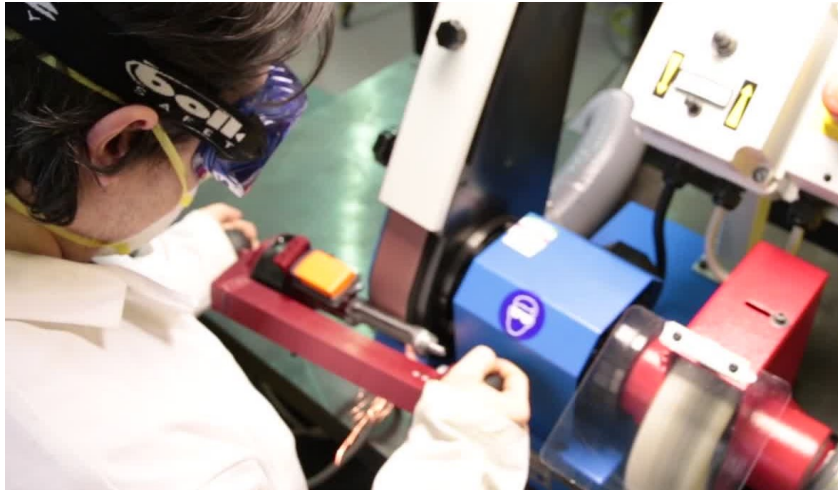
Figure 8.1: Capture of manual polishing parameters with the fixture
