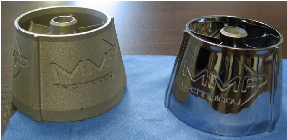
Figure 2.1: Example of an aeronautical workpiece before (left) and after (right) finishing process
