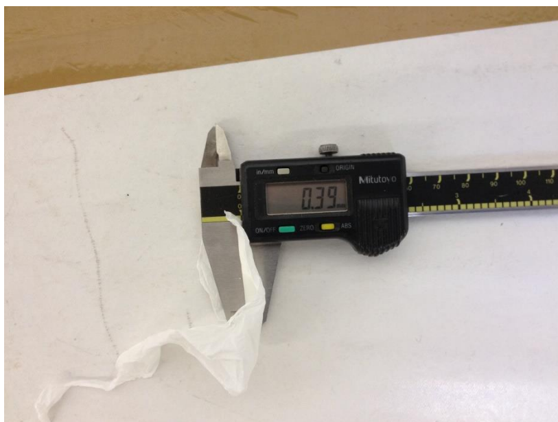
Figure 3.2. Measurement of electrospun mat thickness.
