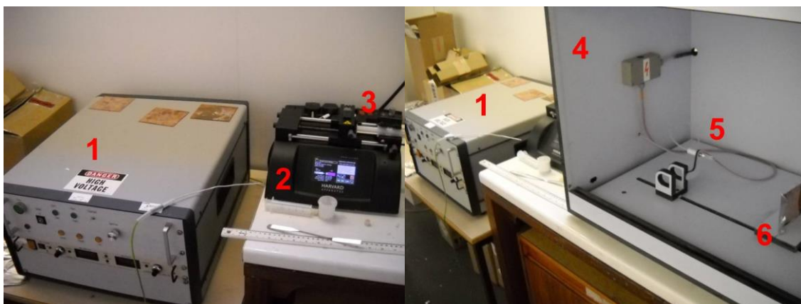
Figure 3.1. Pictures of the electrospinning set-up used for the experiments. The numbers in the pictures represent parts of the rig. 1) High voltage power supply, 2) Pump, 3) Syringe, 4) Ventilated chamber, 5) Metallic needle, 6) Collector.
