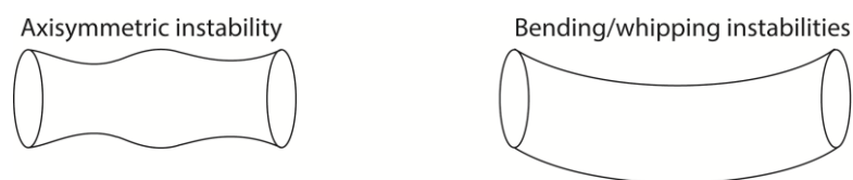
Figure 2.7 - (a) Axisymmetric and (b) non-axisymmetric instabilities in a fluid jet in an external electric field.
