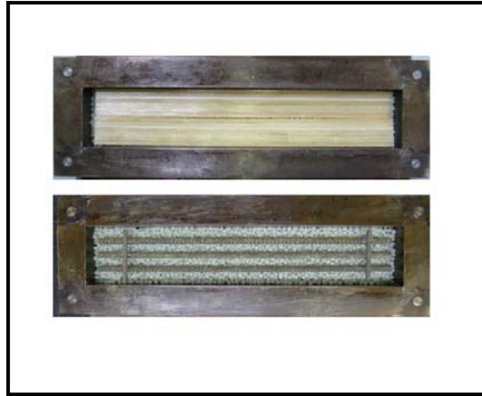
Figure 1 Configuration of glass ribbon (upper) and glass rods (lower image) in the mould.
