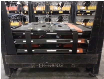
Figure 2 RTIs comprising of a rack and separators with RFID tags attached
