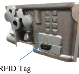
Figure 2. Cylinder Head with attached RFID tag
