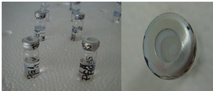
Picture 2.4 Side and top view of the permeation sources, showing vial, PDMS membrane and cap.
