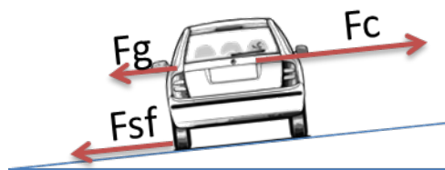
Figure 2 Forces related to the mechanism of skidding
