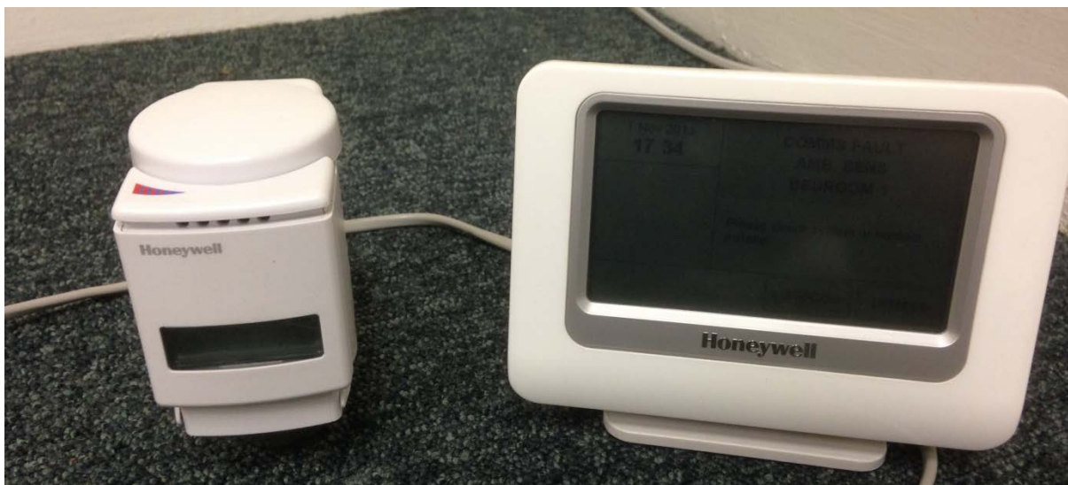
Figure 2-13: Honeywell's Evohome system components including PTRV and central controller
