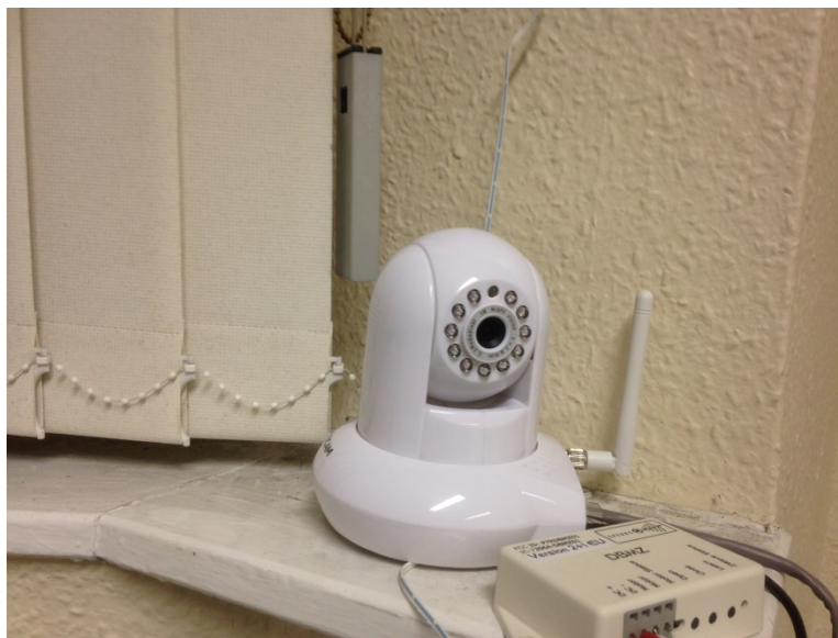
Figure 3-13: IP camera which was used in the living room of a test house to check the operation of synthetic occupancy devices
