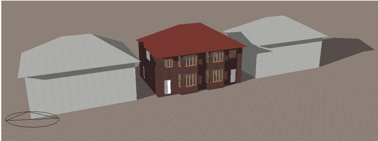
Figure 5-2 View of the LMP1930 test house model with the effect of shading from the neighbour blocks (15 March at 16:00)
