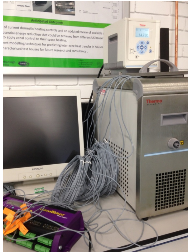
Figure 4-4: The calibration of U type thermistors using water bath calibrator
