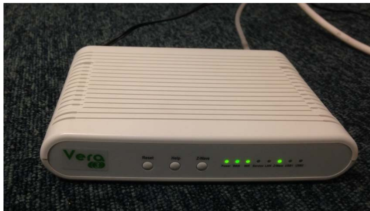
Figure 3-9: Z-wave smart home controller used in each house for synthetic occupancy during the HT1 and HT2
