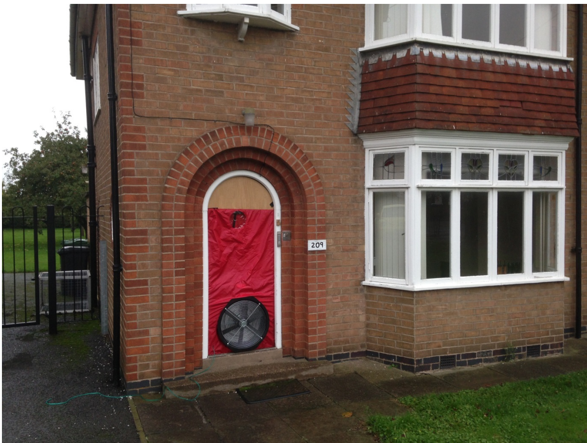
Figure 3-14: The blower door tests set up during the test in House 1
