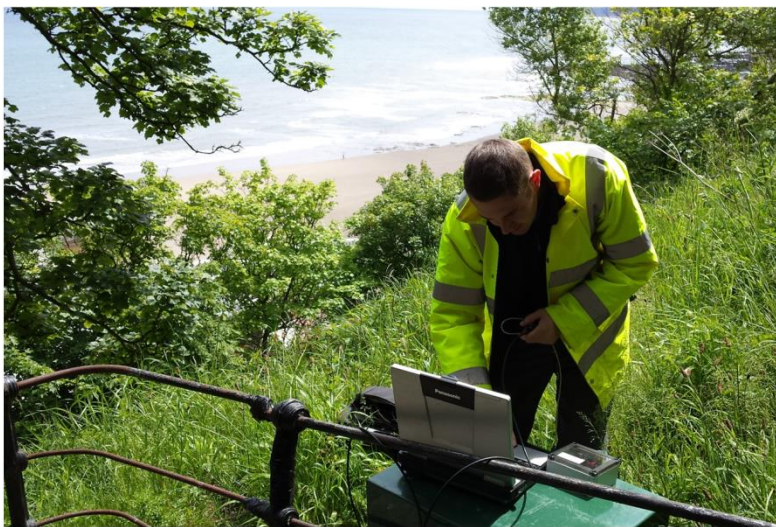
Figure 8. Downloading data from the AE instrumentation at the Scarborough coastal slope
