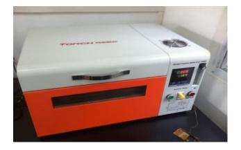
Fig. 4. 7. The reflow oven
