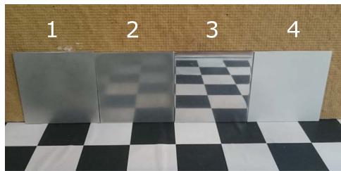
Fig. 2. Photograph of samples. The reflection of the checkerboard pattern on the samples demonstrates their relative surface finish.
