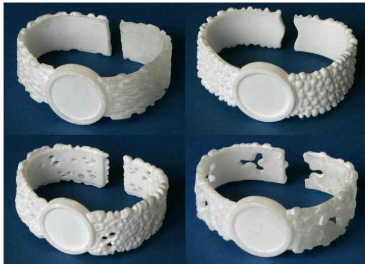
Figure 6. Models produced using multi-jet printing
