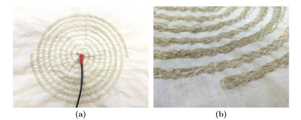
**Figure 5.23** Picture of the fabricated spiral antenna operating from 0.3 GHz to 3 GHz. (a) Top view, (b) zoomed view.
