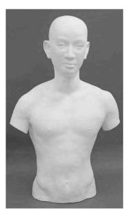
Figure A.5 Realistic human-torso phantom (agar-based solid phantom).
