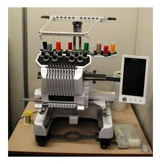
**Figure 5.8** Embroidery machine at Loughborough University used for the fabrication of textile wearable antennas.
