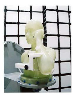
**Figure A.4** A multipostural real-shaped liquid body phantom developed by Ogawa in Panasonic, Japan.
