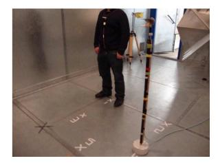
Figure 1.15 Reverberation chamber measurement of textile antenna efficiency on a real human body [51].
