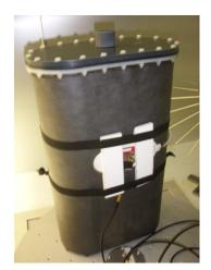
Figure 1.17 Wearable antennas characterisation on a custom made oval torso phantom [60].
