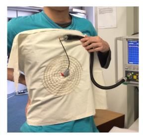
Figure 5.25 Measurement setup of the embroidered spiral antenna on a real human body.
