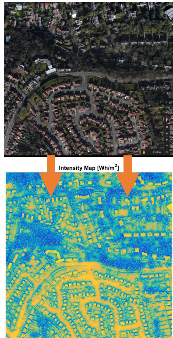
Figure 7: Net annual solar irradiation collection for each pixel in a 0.25 km 2 LiDAR map of Prestwich, UK, for 2014 using interpolated Met Office irradiation data
