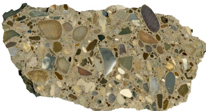
Figure 1: Thin section of demolition concrete for petrographic analysis [46]
