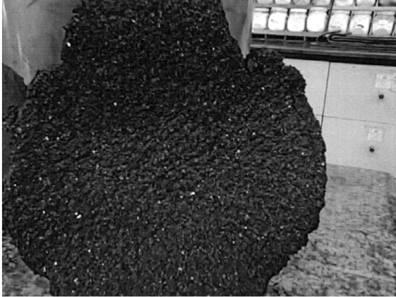
Figure 3. Devulcanized compound B-3 after removal from the autoclave and subsequent drying in air for 24 h.
