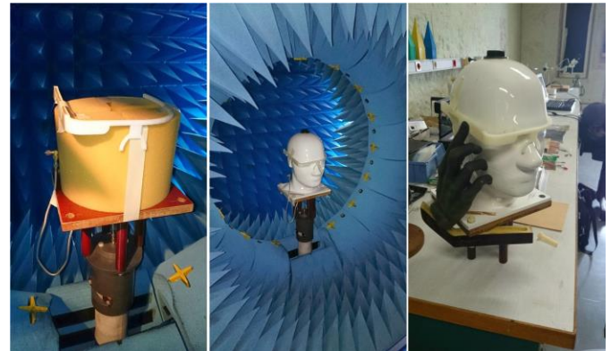
Fig. 8. Measurement configurations for the three targeted use-cases: "free space" using foam spacer (left); "with SAM head" (center) and "with SAM head and phantom hand" (right)
