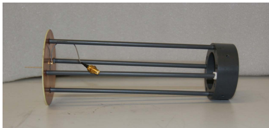
Fig.5. Monopole antenna mounted on the support pole.
