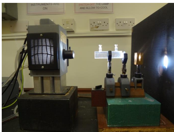
Picture 5. 300W Xenon arc lamp
