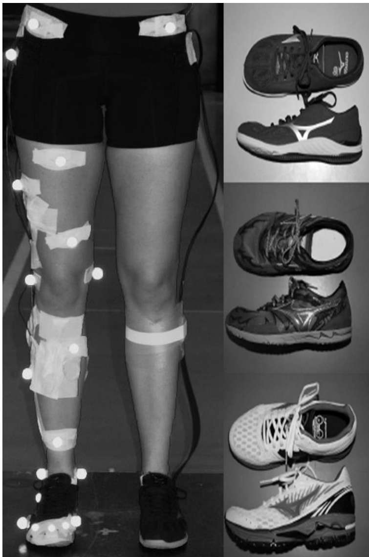
433 Figure 1. Marker set-up including anterior and posterior superior iliac spine (RASI, 434 LASI, RPSI, LPSI), thigh (three markers), shank (three markers), fifth 435 metatarsal, forefoot (three markers) and hindfoot (three markers). Additional 436 markers were added on the right greater trochanter, lateral and medial femoral 437 epicondyles, lateral and medial malleoli, first metatarsal during static trials in 438 order to identify joint centres. The running shoes used in this study were Be 439 (top), Universe (middle) and Rider (bottom).
