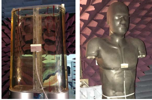
Fig. 6 a) Simulation setups for far field evaluation: HOCS, Full Liquid and Voxel Phantom and b) Measurement setups for far field evaluation: Horizontal printed dipole antenna mounted on a HOCS and on a solid anthropomorphic torso phantom
