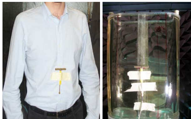
Fig.3 Measurements setup of the 2GHz sleeved balanced dipole antenna mounted on the middle of the torso of a volunteer and of the HOCS torso phantom
