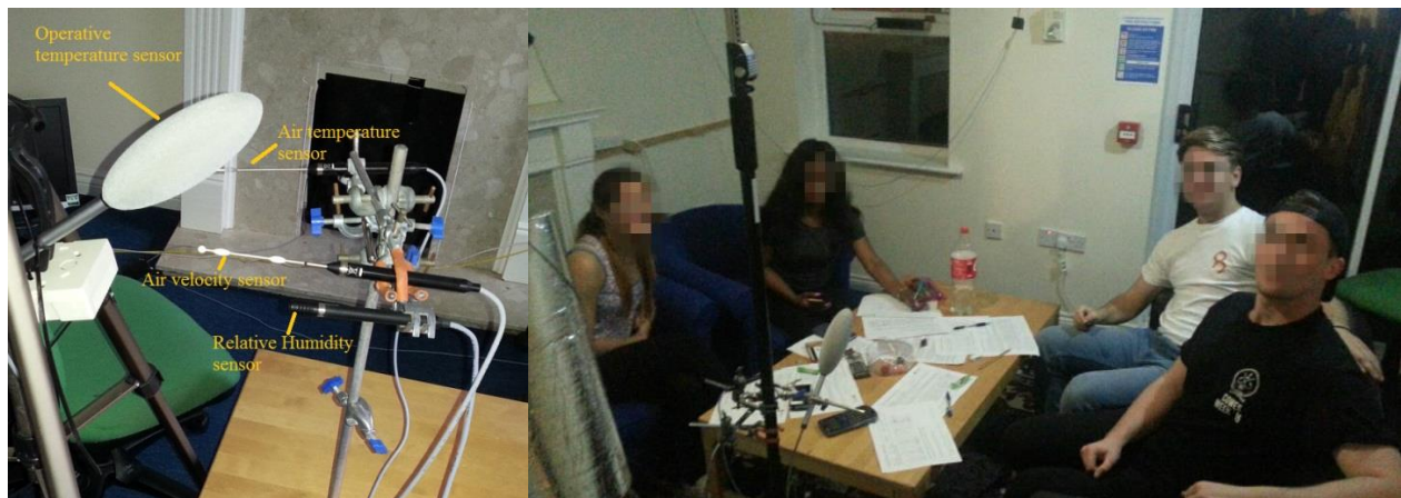
Figure 2 Left: Equipment arrangement (operative temperature sensor height 0.8m, Air Temperature sensor and Speed sensor height 0.6m and Relative humidity sensor height 0.5m). Right: Typical four participants filling in surveys
