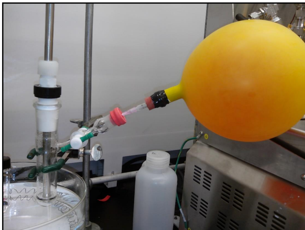
Figure 5.5.-Experimental set up for the cyclic carboxylation reaction of epichlorohydrin with \text{CO}_2 and TBAI.
