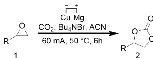
Scheme 1.1.- Electro-synthesis of carbonates from epoxides under mild conditions. 1
