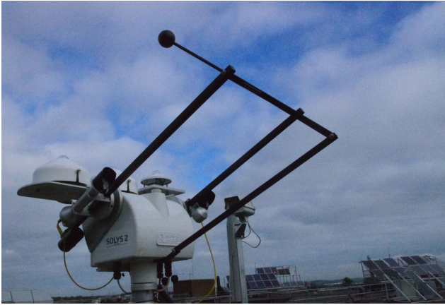
Fig. 1 Photograph showing instruments for measurement of horizontal, beam and diffuse irradiance measurement on a Solys2 sun tracker at Loughborough University
