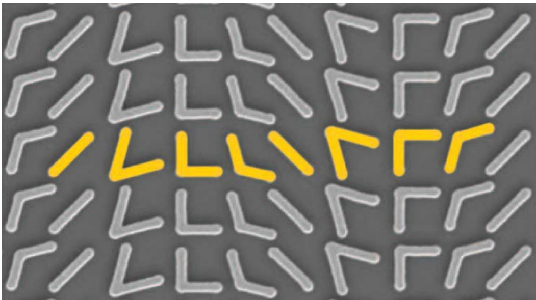
Figure 4-4: A metasurface with sub-wavelength v-shaped anisotropic scatterers. The orientation of the scatterers has been varied in order to gain a full phase control of the wavefront [32]
