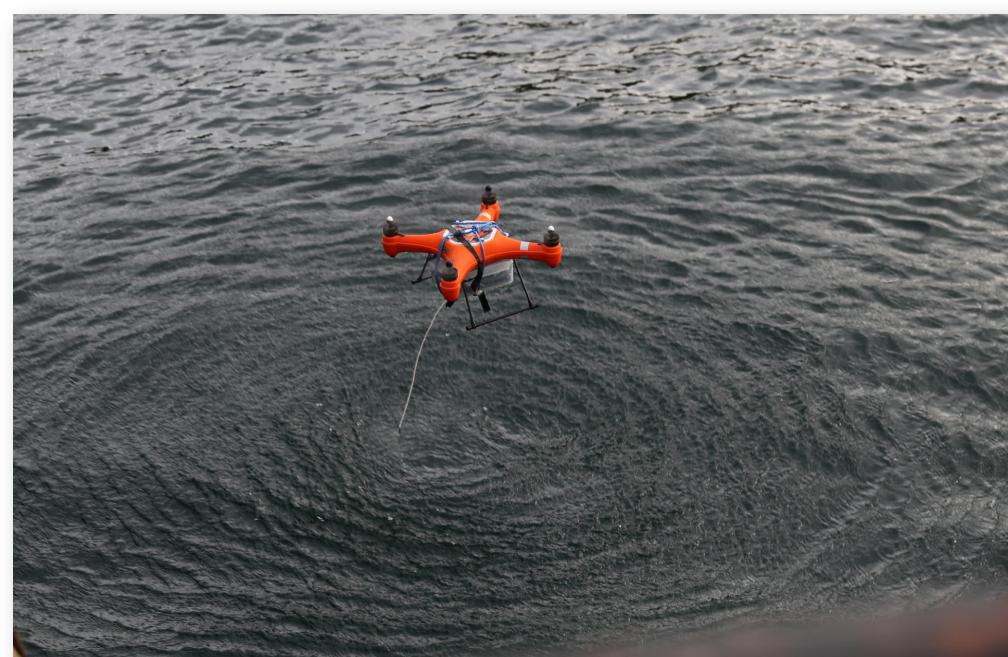
Figure 2b) In-flight deployment of hydrophone system
