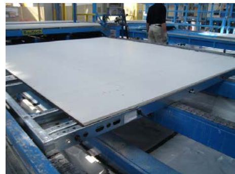
Figure H.4: Wall panel with first layer of board fitted, prior to taping the board joints
