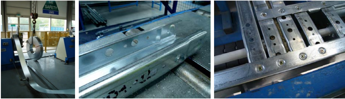
Figure H.1 (left): Rolls of light gauge galvanized steel ready for cold-forming in the factory
