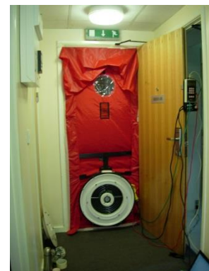
Figure 3.11: Minneapolis blower door model 3 during testing
