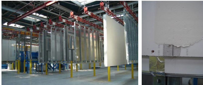
Figure H.8 (left): Wall and ceiling panels hanging at the end of the paint line, already painted
