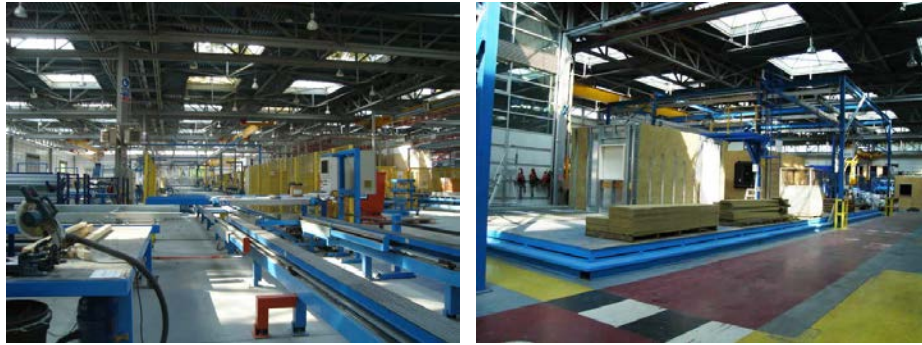
Figure 4.3 (left): [redacted] factory floor, showing panel framing machine Figure 4.4 (right): [redacted] factory floor, showing module near completion
