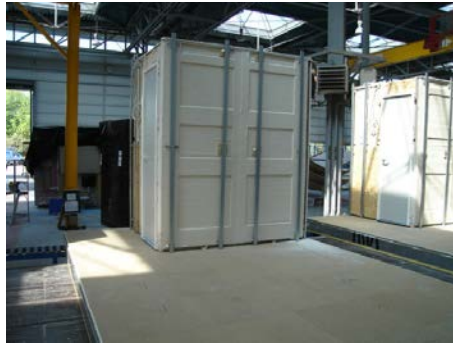
Figure H.12 (left): Shower pod ready to be lifted onto floor panel
