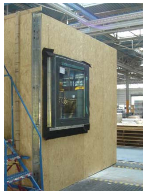
Figure 4.12 (far left): Modular windows with steel angles and DPC fitted prior to delivery to [REDACTED] factory
