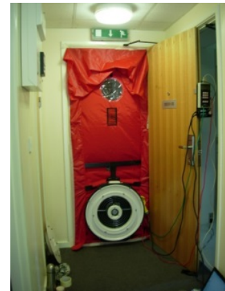
Figure 7.2: Blower door equipment setup in main entrance door of test flat
