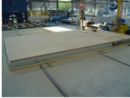
Figure H.10 (left): Floor panel with rigid insulation fitted to underside, and space heating pipework fitted
