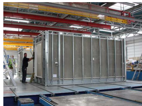
Figure 4.5: [redacted] factory floor, showing four-sided module during manufacture [redacted] 2012]
