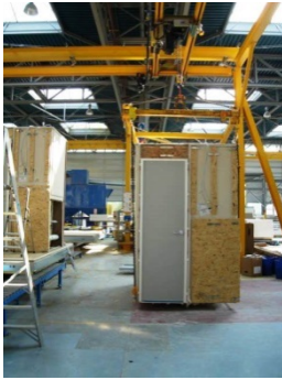
Figure H.12 (left): Shower pod ready to be lifted onto floor panel
