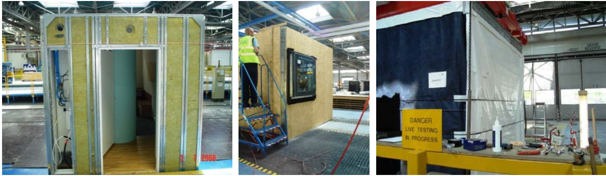
Figure H.24 (left): Factory photo showing fire insulation fitted between wall studs [REDACTED] 2012]
