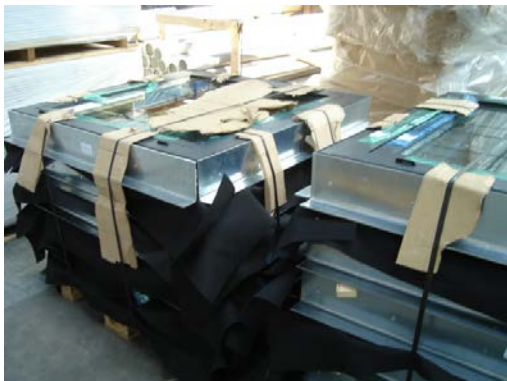
Figure 4.12 (far left): Modular windows with steel angles and DPC fitted prior to delivery to [REDACTED] factory
