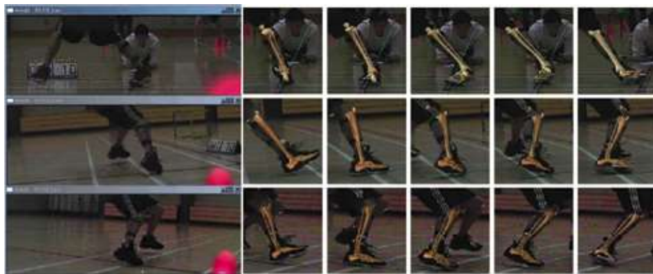
Figure 4.3: An accidental ankle sprain case which happened during a sports shoe stability test in a laboratory.
