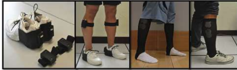
Figure 4.8: The first prototype as two pairs of detachable parts at the heel counter and the shank, and the second prototype as a pair of sport leggings.
