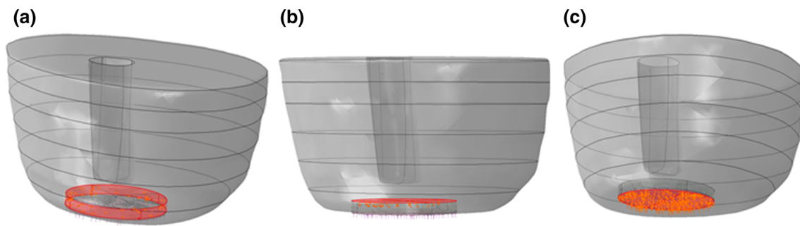
Fig. 4 Schematic representation of simultaneously applied loading conditions for macro-scale model: The red areas represent the affected surface of tissue or filler, and orange arrows indicate the direction of
