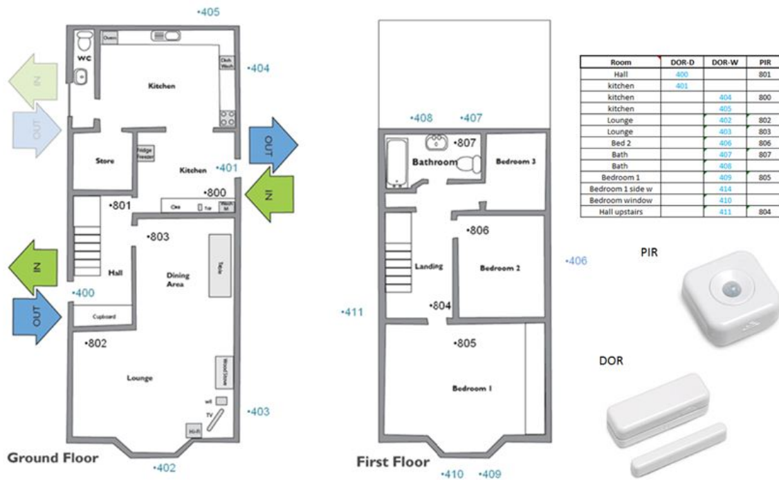
Figure 3.5: PIR and DOR sensors sample location
