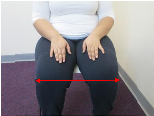
Figure 5.1 Knee Splay. Measured horizontally between the outer borders of the knees in preferred comfortable posture.
