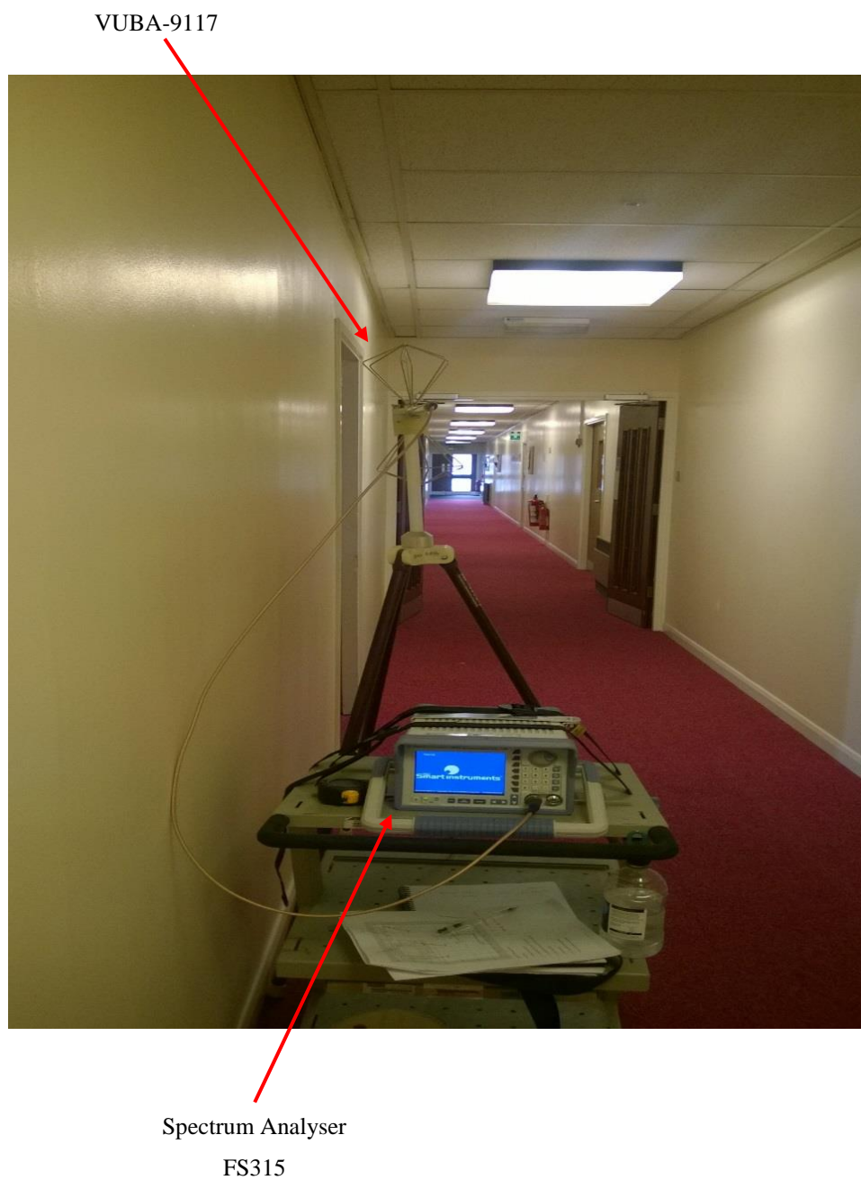
Figure 5.36. Photographs of receiver system placed at different locations throughout the building.
