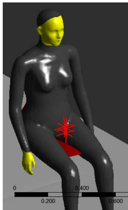
Figure 6-8: Points of maximum residuals located near to the chair region shown as red cross points.
