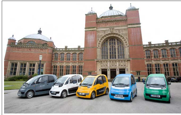
Figure 1.6: The Microcab H4 FCHEVs at the University of Birmingham - Kendall et al. [4]
