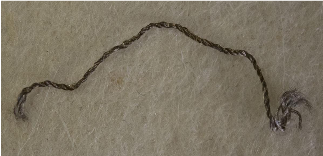
Figure 5.22 Cutoff section of the washed thread from the stitched transmission line
