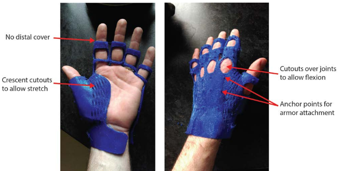
Figure 4: Iteration 2 prototype - full glove custom-made for hand therapist for evaluation
