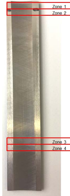
Figure 2: Liner sample prepared for AFM measurement with the defined Zones 1-4
