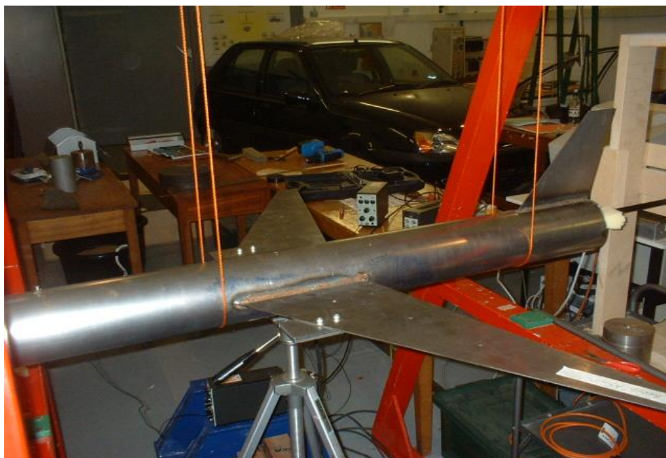
Fig. 3. The manufactured reduced-scale aircraft model supported by suspensions
