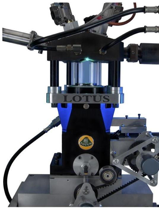
Figure 1. Optically accessible engine - Lotus SCORE
