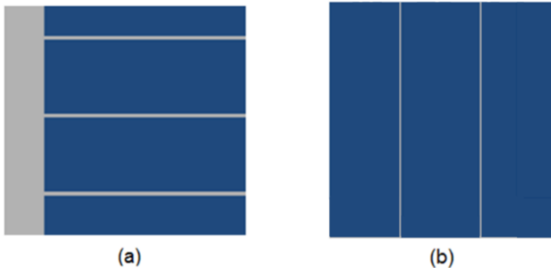
Figure 4.2. (a) The layout of the front contact layer of the c-Si virtual sample. (b) The layout of the 3 cell thin film virtual device.
