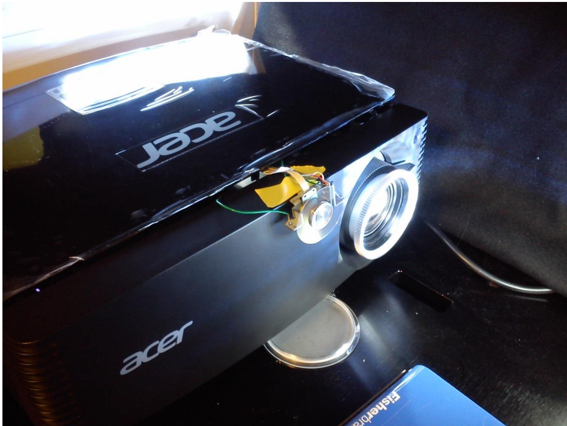
Figure 6.8. The DLP projector operating after the removal of the colour wheel from the light path.
