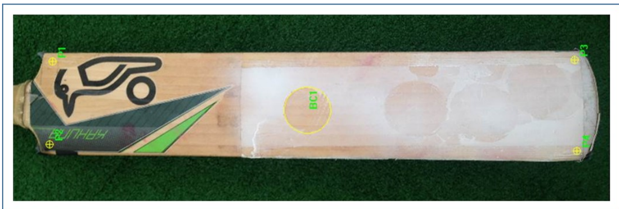
Figure 4. Impact location measurements derived from the impression imparted to a fine powder coating on the bat face.
