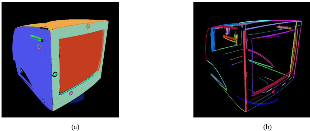
Figure 3. (a) Surface feature model and (b) curve feature model of a CRT monitor model.
