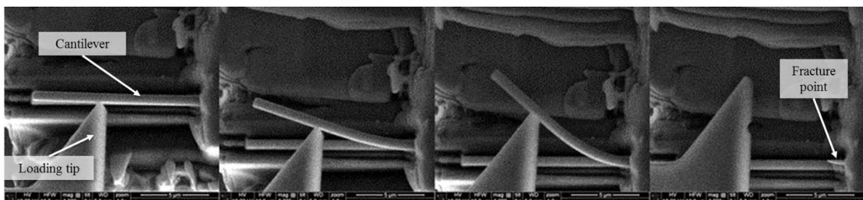
**Figure 1.** micro bend testing in progress left to right showing deformation to failure
