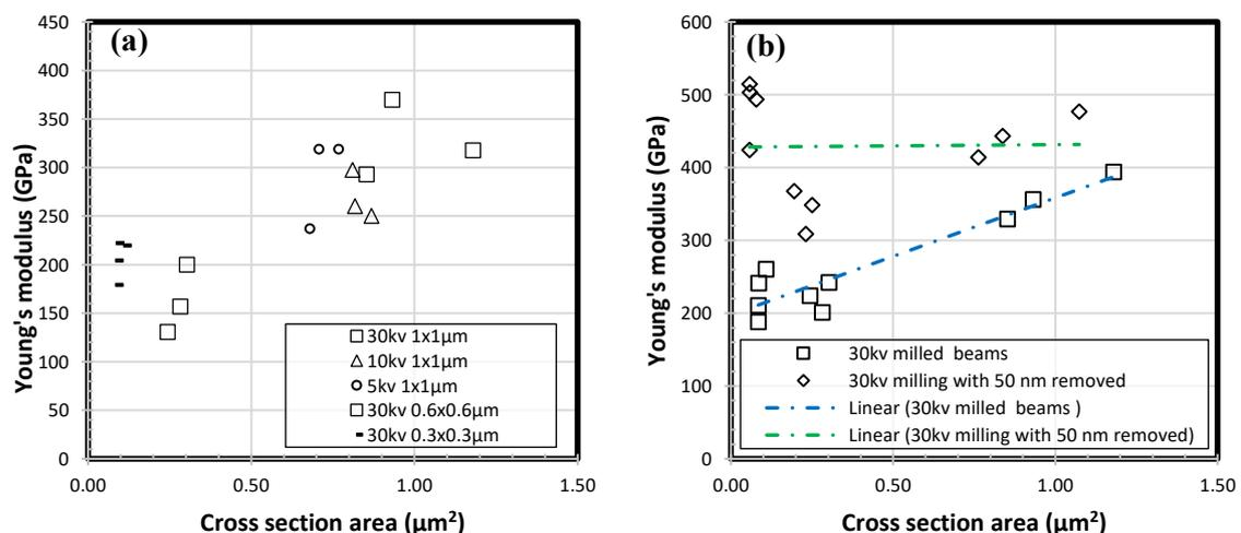
**Figure 2.** (a) micro bend test results modulus against cross section (b) adjusted micro bend tests data with original 30 kV data and beams with 50 nm removed from breadth and width
