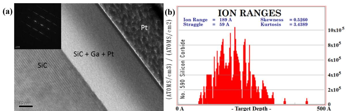
**Figure 3** (a) shows HRTEM image of silicon carbide surface with the amorphous layer and platinum protective coating. (b) SRIM simulation of 30 kV gallium ion implantation distribution in silicon carbide
