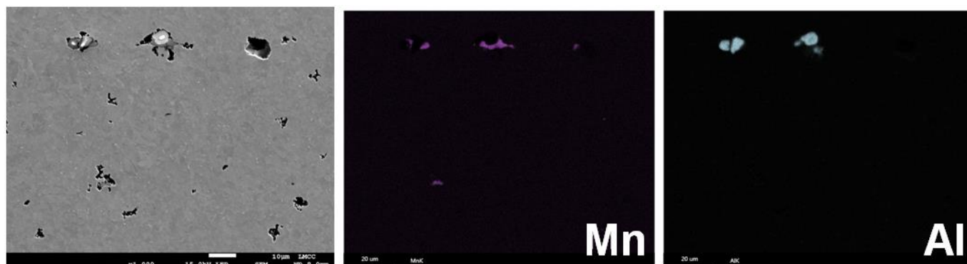
Figure 10. SEM-EDS Analysis for Damage at Inclusions in Sample RNT-B2-2 (parent Metal B2) and for Al and Mn
