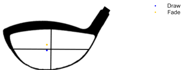
Figure 8-1: Group-level significant difference in vertical impact location for driver draw versus fade trajectories.
