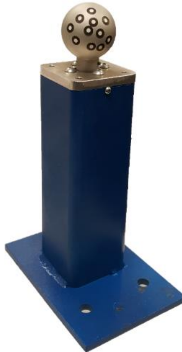
Figure 3-15: Purpose-built spinning device designed to validate the GOM method spin rate calculations.
