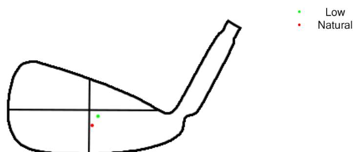
Figure 8-2: Significantly different vertical impact location of golfer five's low versus natural trajectories.
