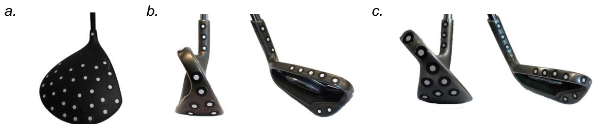
Figure 3-9: GOM marker placement on a. the driver; b. the 7-iron and c. the utility wedge.
