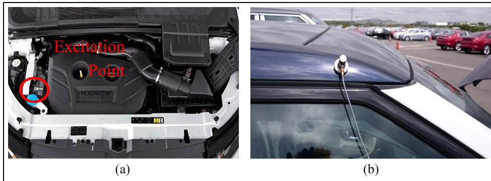
Figure 2(a). The photo shows the bonnet interior of a Range Rover Evoque, with the site at which the vehicle is excited with the impact hammer. (b) The measurement response position above the upper A-pillar. The accelerometers were held on with the use of a magnet.
