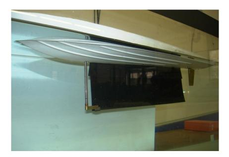
Fig. 4 Underwater view of the mono-hull model boat with the assembled propulsive rubber plate (Krylov et al., 2010).
