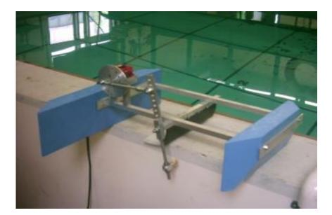
Fig. 3 View of the model catamaran with a propulsive rubber plate before testing in the experimental pool (Krylov et al, 2007a,b).
